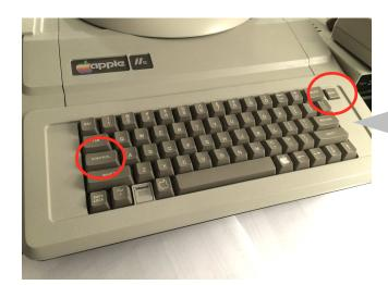
To start over, press <CONTROL> <RESET> or just turn the computer off and back on.
