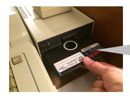
Hold the disk by the label and insert it into the disk drive. Close the door.
